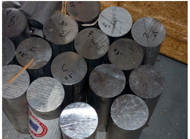
This round stock is used for various parts, including the rear panel of the Carmel's cabinet.
