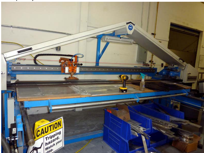
This machine finishes the outer cabinet walls.
